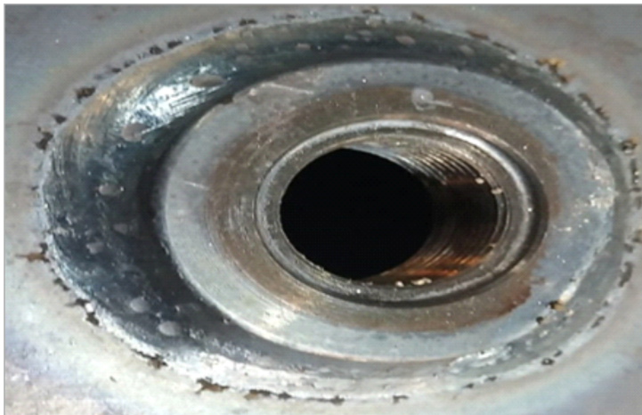
Moisture in flux leads to pockmarks
